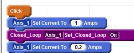
The current setting indicated above the block turning on closed loop should be a high value to insure a stable accurate initialization. After turning on closed loop the current can be reduced.
