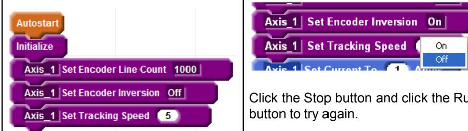
These adjust closed loop settings. Click on the encoder line count field and set for the encoder you are using. Tracking Speed establishes how fast a lagging motor will try to catch up. This speed must be higher than the fastest speed you intend to use but can be set faster.
